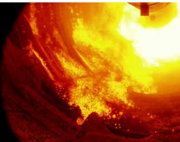
Burner zone in a rotary kiln with cement clinker
